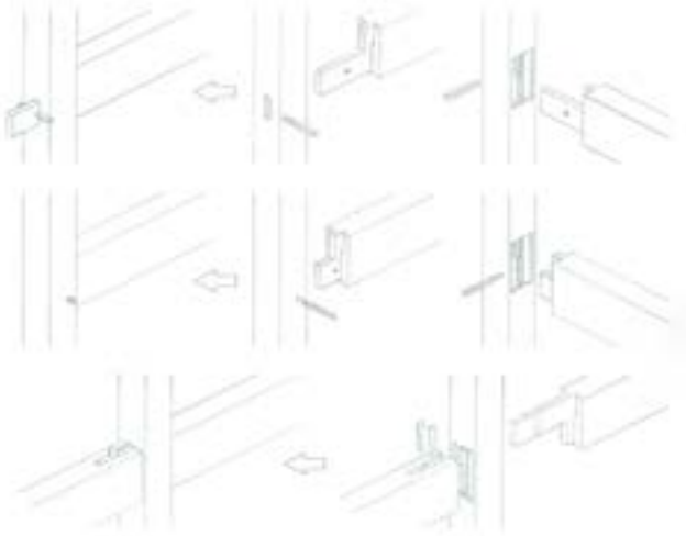
(Figure 2) Shikuchi joints used for sashigamoi, ashigatame, etc. Konehozo-hanajime/Oire, Konehozo-komisenjime/Oire, Konehozo-shachisenjime/Oire | (Figura 2) Juntas Shikuchi utilizadas para sashigamoi, ashigatame, etc. Konehozo-hanajime/Oire, Konehozo-komisenjime/Oire, Konehozo-shachisenjime/Oire | (Figura 2) Juntas Shikuchi usadas nos sashigamoi, ashigatame, etc. Konehozo-hanajime/Oire, Konehozo-komisenjime/Oire, Konehozo-shachisenjime/Oire
