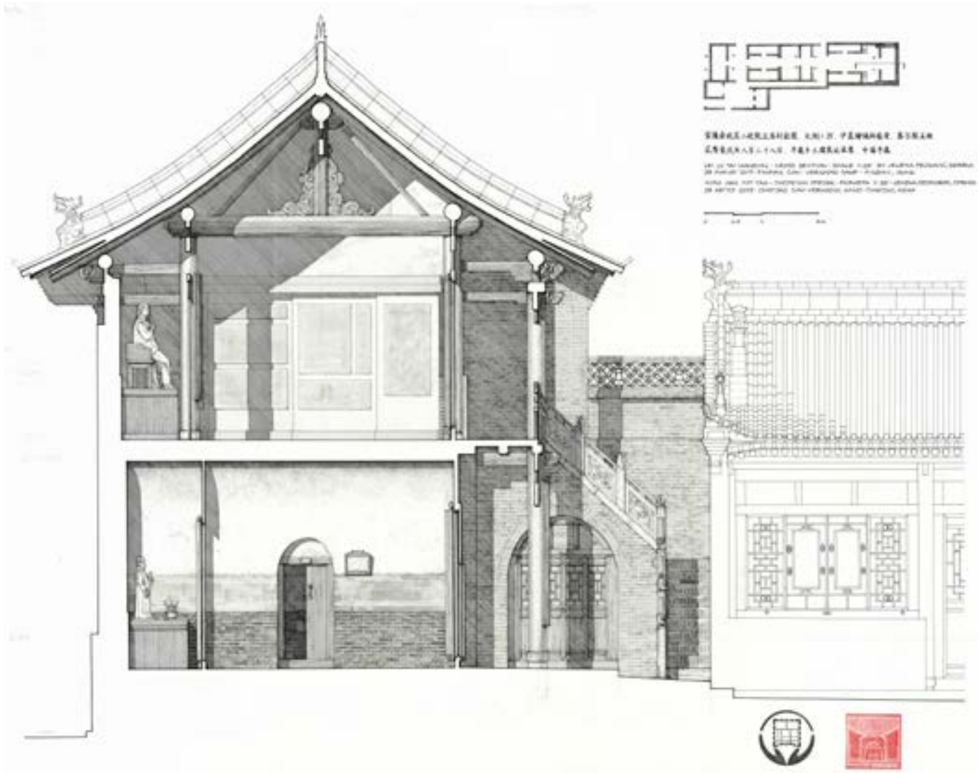
Cross section of the Lei Lv Tai Mansion, Pingyao, China. Original scale 1:25
