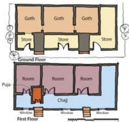
Figure 21. Single line sketch plan of first typology of Barpatiya dwelling
